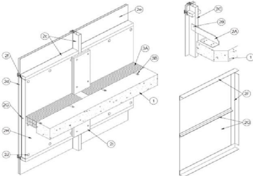
**1. Floor Assembly-** Min 8 in. (203 mm) reinforced normal weight (125-150 pcf or 2000-2400 kg/m<sup>3</sup>) structural concrete.
