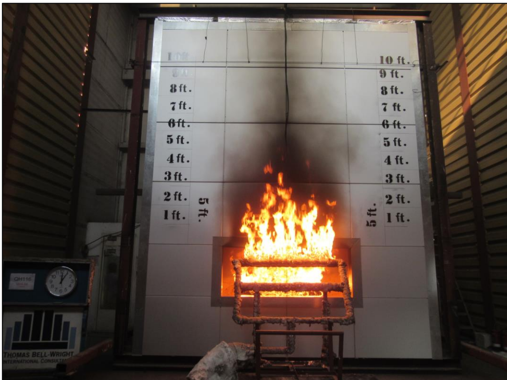
Picture B: At 5 minutes from the start of the test the window burner was ignited.
