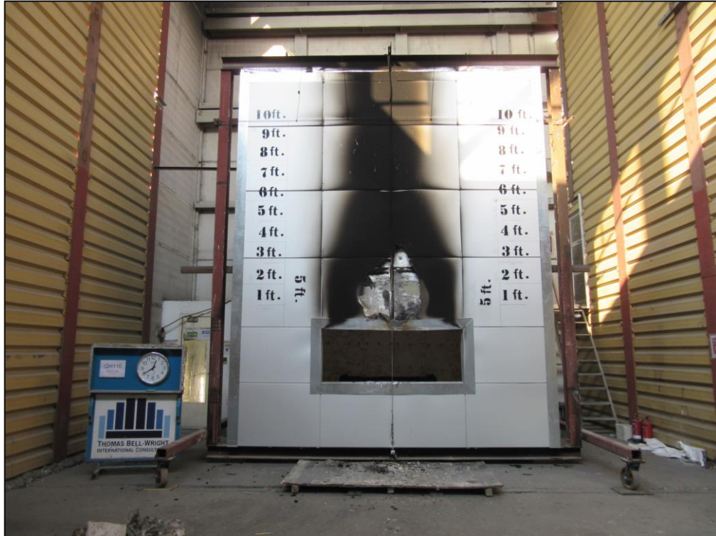
Picture E: Specimen at 40 minutes. End of the observation period and NFPA 285 test.
