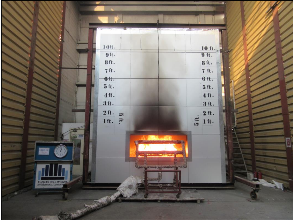
Picture A: Room burner was ignited. Start of the test.
